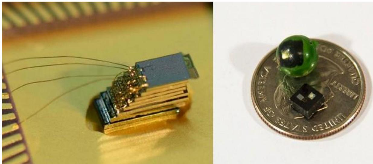
Measuring just 3 mm across (left), this device contains batteries, sensors, and other components needed to autonomously collect, store, and report temperature and pressure measurements. Encased in a polymer coating (right, black) and then in an outer coating to control buoyancy (right, green), this data logger is designed to travel safely through an underground oil reservoir.
